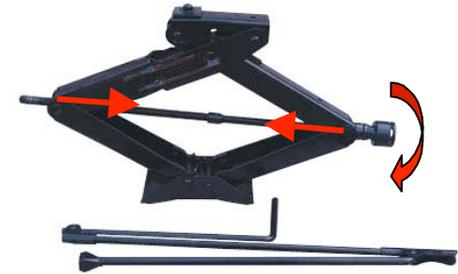
Rotating the screw shaft on the scissors jack causes the two sides to move towards the center. This is a classic example of using a screw to change rotary motion into linear motion.
