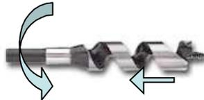
makes the chips move up the bit.
